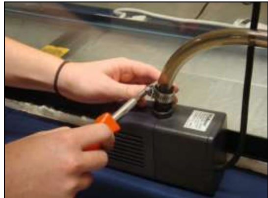
Attach vinyl tubing to the hose barb with a SS hose clamp
