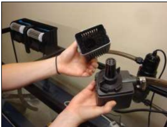
Pop off the top of the pump to locate the pre-filter
